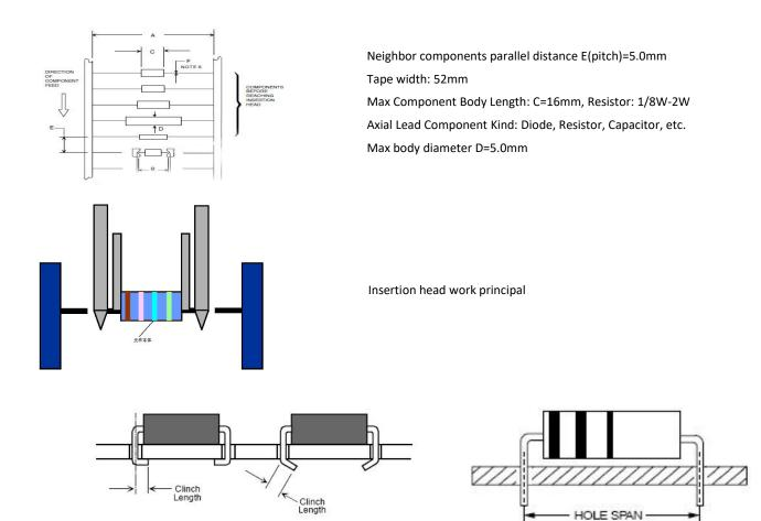
Hole Span: 5~20mm
